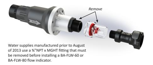
Wrap threads 2.5 times with a 6" length of .5" PTFE (Teflon style) tape prior to threading into flow indicator. Tape should be wrapped in a clockwise direction and should not overlap or cover the inlet of the coupler. Coupler should be hand tightened only. (BA-FLW-60 only)
