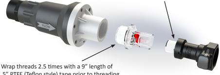
.5" PTFE (Teflon style) tape prior to threading into regulator. Tape should be wrapped in a clockwise direction and should not overlap or cover the inlet of the flow barrel. Flow indicator should be hand tightened only.
